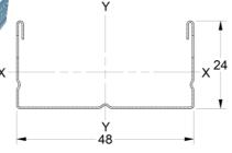
GypFrame® PRMA Master Section is a common channel for ceiling frame. It is used as furring channel as well as main runner in the ceiling. It includes slots to assist fixing furring channel to main runner using connecting bracket.
